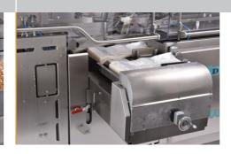
Self-cleaning vacuum filter – "Jet Filter": The filter inserts are cleaned via cyclic bursts of compressed air.
