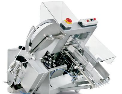
Product guides that can be adjusted quickly and without tools allow for short set-up times.
