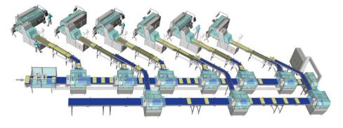
EC 130 + SL 20 + SFB + DT The EC 130 is ideally suited for linking with a Selectra slicing machine or a GS 60 reciprocate slicing machine.
