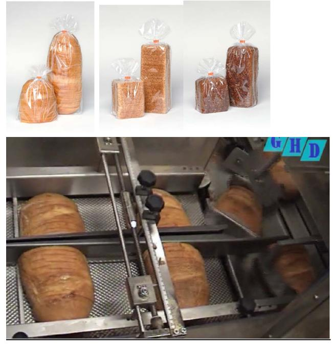
GBK turning  $180^{\circ}$  '(from left to right slicing, separation, turning of one ½ loaf, feeding into bagger GBK upright slices)
